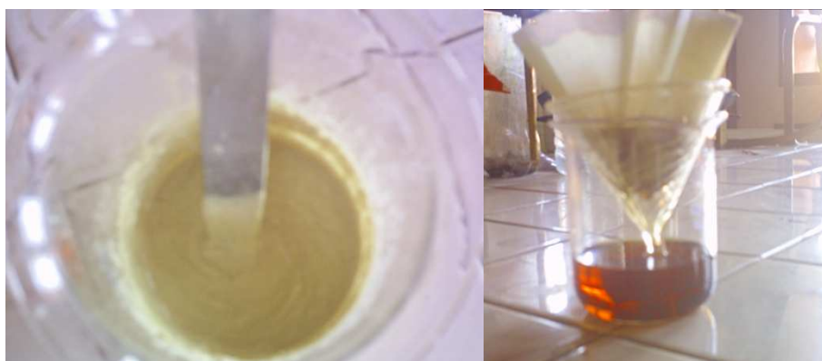
Figure 10: ferric Sulphate before the solubilizations (on the left) and after solubilizations and filtration (on the right)
